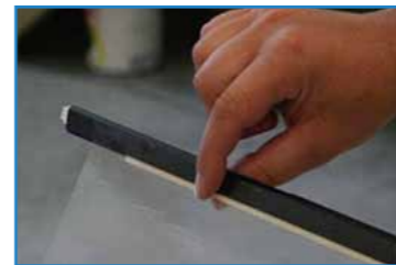
Transparent touch sensing foil
